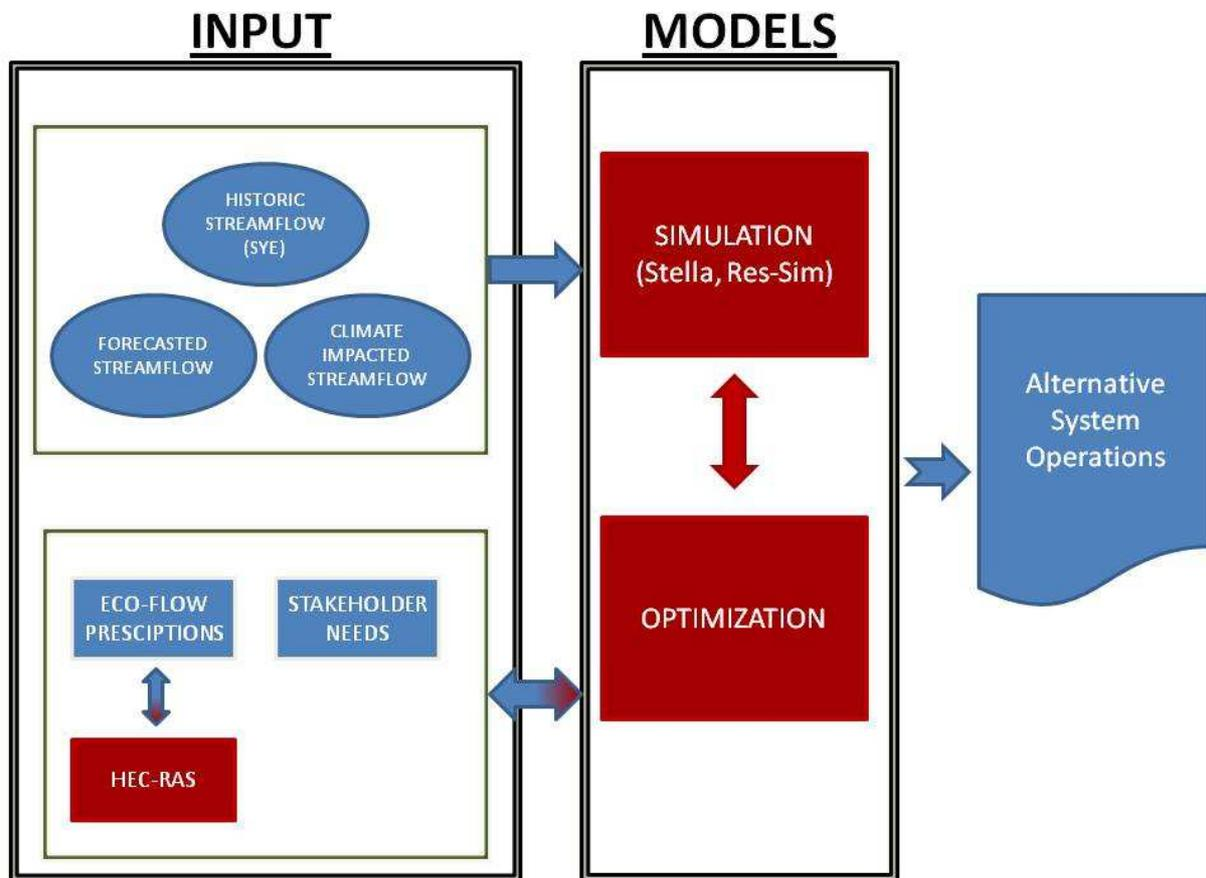
**Figure 1.** Basic structure of multi-agency water management decision support system for the Connecticut River basin, which includes an optimization routine with environmental flow targets.
